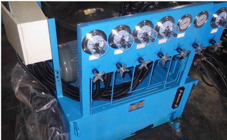
▲ Hydraulic power supply after decontamination
